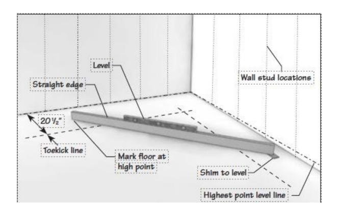
Over time a house settles, and the floor can develop a subtle slope. To ensure a level installation throughout the kitchen, you'll need to identify the high spot on the floor and start your installation at that point. You can always place shims underneath a cabinet to make it level, which is much easier than cutting it down to level with the floor.
